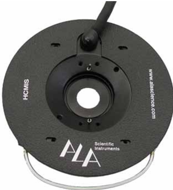
HCMIS shown with gas ports and magnetic mounting plate installed at top and MS-502 chamber in middle
