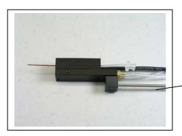
The HCPC can be mounted on a magnetic base with a swivel as pictured above, or via mounting rod (3.2mm 1/8<sup>th</sup> in.) Rods are about 10cm long.
