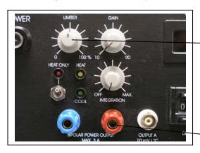
Notice the limiter on the PTC is set with the line at 12 o'clock. This will keep the voltage at just under 7 volts, in the safe zone. The limiter is active whenever the unit is in the control mode. It prevents the PTC from burning out the HCPC when full power is called for.
