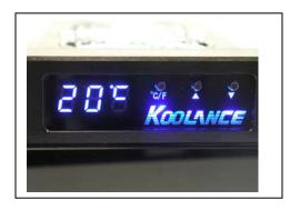
The front panel will display the temperature. There are three buttons. One will switch between F and C for the temperature monitor, the other buttons will allow manual adjustment of the fan speed (9 speeds) or select automatic. Typically the lowest fan speed is adequate for the HCPC even at 0°C set point. Adjust as necessary, warmer environments may require more air flow to get enough heat transfer. There is no pump speed adjustment.
