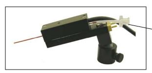
The input of the HCPC is silicone tube equipped with a female Luer connection. The ID of the silicone tube is about 1mm so most ALA manifolds can be connected directly to the tubing if the Luer is removed. Otherwise your perfusion system can be coupled to the HCPC with a male Luer.
