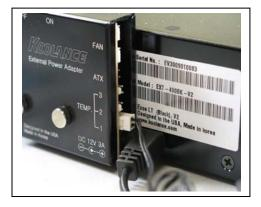
Since CPU coolers are usually powered through the power supply of the computer, this one requires a 12V power adapter with wall transformer. The transformer is universal so it can work anywhere in the world. The power switch is located on top of the power module shown in the photo above.
