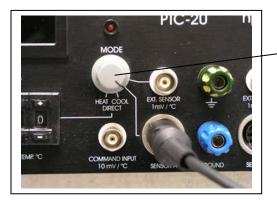
Remember that when the mode switch is set to Direct, DC Voltage will be supplied to the HCPC. The amount will be set by the pin-wheels. The number you set represents a percentage of the full power that can be applied. The Limiter is by-passed in Direct mode, so do not set the value at more than 500, as this represents 50% of 14 Volts, or 7 Volts.
