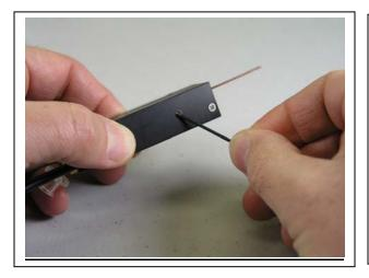
On top of the unit is a small set screw, the thread is 4-40 (Use .050 standard Allen wrench). It can be used to loosen and tighten the seal of the perfusion pathway. Typically it is factory set to a tight position which limits the amount of fluid that can be in the fluid path. This lowers the dead volume, but slows the flow rate. This screw can be loosened up to one full turn to increase the flow rate and lower resistance to flow. Just be sure not to loosen it to the point of leaking.
