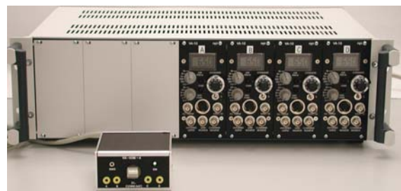
EPMS rack housing w/4 VA-10M modules and single headstage
